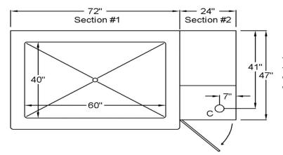
Temperature......40°F to 70°F Tank Capacity......270 gal. Weight (Filled)......3,755 lb. Weight (Empty)......1,500 lb.
